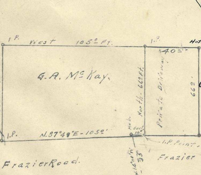
Map of George A. McKay tract located in N/2 of N.E/4 Sec. 12 Twp. 5 S., Range 33 E.W.M. Surveyed, staked & platted Nov. 1952 by W.E.O. Criger. Scale: 1" = 40'
