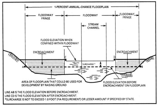
**Figure 1. Floodway Schematic**
